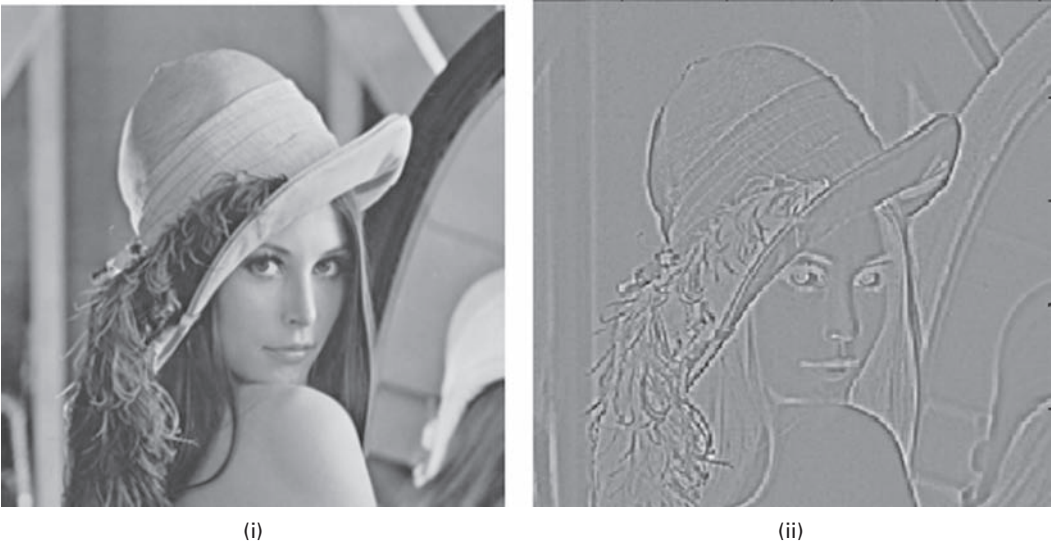
Figure 6.34 (i) Original (noiseless) image and (ii) result of Laplacian of a Gaussian operation.
