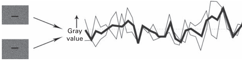
Figure 6.1 Noisy CT images of a water phantom, with a profile from each (solid lines) and the mean of the two profiles (thick solid line).
