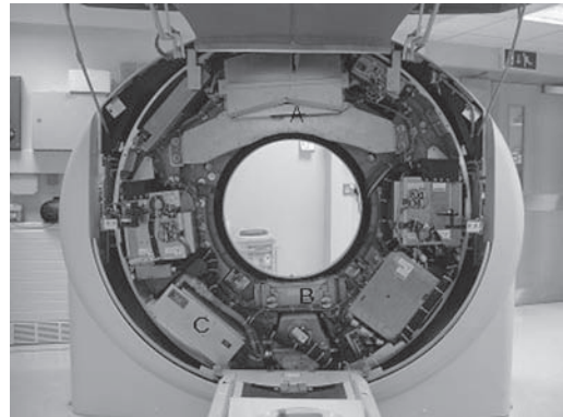
Figure 3.25 (i) Outside view of third-generation CT scanner showing the patient table and gantry aperture. (ii) When the cover is removed, the x-ray tube and the arc of detectors can be seen. The gantry holding the x-ray tube and detector rotate around the patient as the data are gathered.
