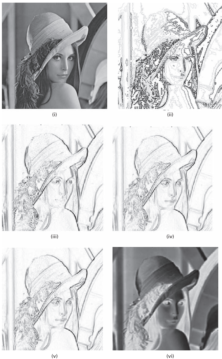
Figure 6.30 (i) Original (noiseless) 256 × 256 image and (ii) its contours. Results of gradient edge detection using (iii) Roberts, (iv) Prewitt, (v) Sobel, and (vi) Frei–Chen operators. See also color plate.
