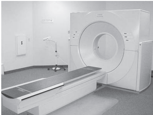
Figure 3.25 (i) Outside view of third-generation CT scanner showing the patient table and gantry aperture. (ii) When the cover is removed, the x-ray tube and the arc of detectors can be seen. The gantry holding the x-ray tube and detector rotate around the patient as the data are gathered.
