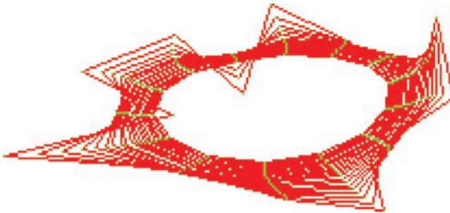
Plate 24 Twenty iterations of a snake (red), starting from an outer contour, moving under an internal elastic function. The trajectories of the control points are shown in green.
