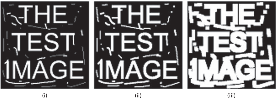
Figure 9.5 (i) Original image; (ii) after a single dilation; (iii) after several dilations.
